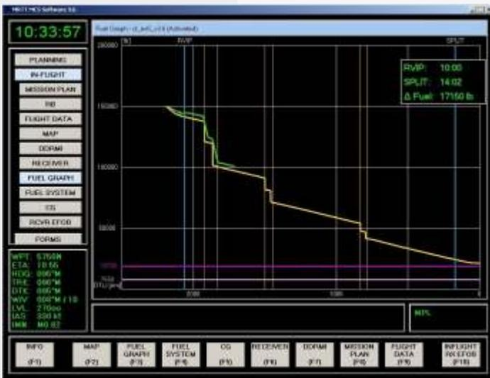
The tanker's onboard fuel is calculated along the trail mission, taking the refueling events into account.
