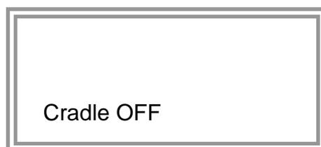
If no external memory is connected or no 24bit address is defined the message "CRADLE OFF" appears. In this case the device is working as "Mode AC only" transponder.
