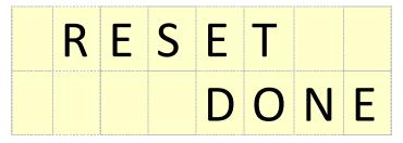
The reset process is activated by pressing the SET button. The reset is confirmed with "DONE" and the transceiver automatically restarted
