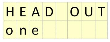
The setting "one" is required when operating the transceiver with an old harness (without extension -S in the cable name). Adjusting the volume of the sidetone during transmission is then carried out via the menu item STL (Sidetone Level) and controls both headphones. The menu item STR is hidden.
