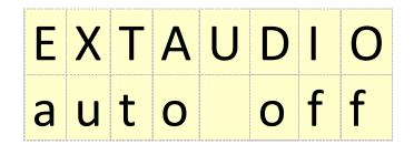
**not RXTX**: The external audio input is automatically deactivated during radio reception or transmit mode. This setting does <u>not</u> use the external audio activity sensing, and therefore can introduce noise when no signal source is connected.
