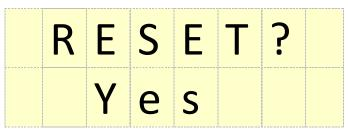
The reset process is activated by pressing the SET button. The reset is confirmed with "DONE" and the transceiver automatically restarted
